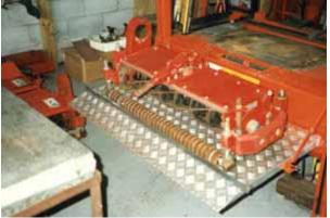
The frame for the table is made of 1.5 X .187 angle with 400lb. load casters. We built it with a shelf that actually held 3 spare greens reels. Moving it was next to impossible so it's now used for misc storage. The setup table and the lift table, both have removable metal stops. With the non-stop interruptions in the shop, just turning around at the wrong time can lead to disaster with a reel rolling off.
